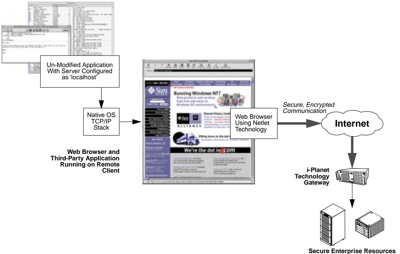
Figure 2 The Netlet, one of the more powerful components of the i-Planet product, enables secure, encrypted communication from un-modified client applications back to servers in the enterprise network.
