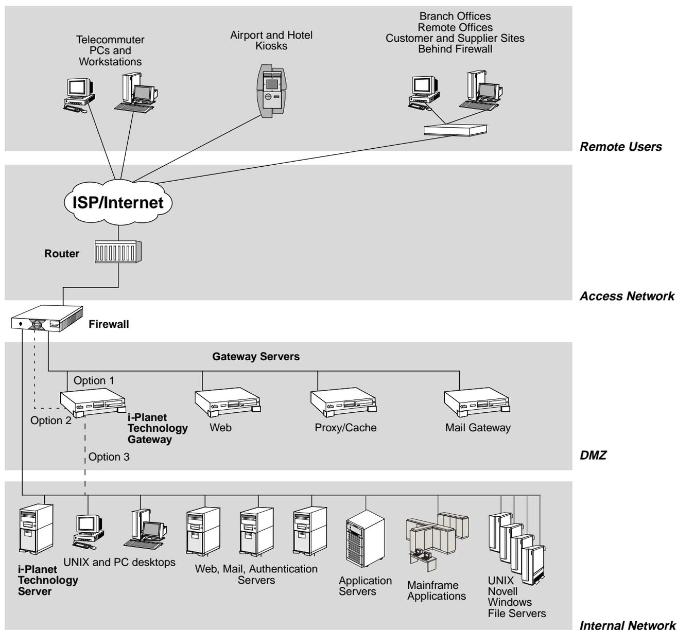
Figure 3 Enterprise configuration of i-Planet software illustrating the gateway located in the DMZ and the server in the organization's internal network.
