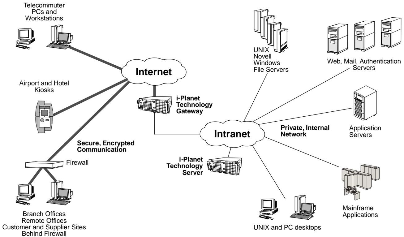
Figure 1 Secure, remote user access is provided by i-Planet software hosted on a gateway and a server platform. Remote users may be located anywhere on the Internet, including behind other corporate firewalls.
