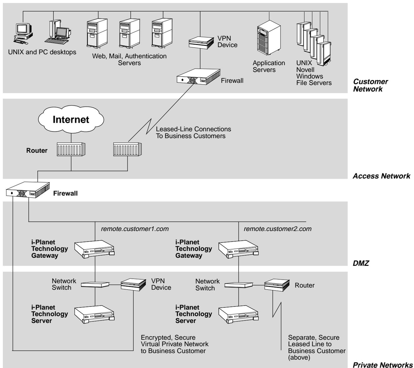
**Figure 4** ISP configuration showing two business customers supported at the ISP site; private traffic to the first customer (left) is routed through a virtual private network into the company's network; private traffic to the second customer (right) is routed via leased line to the company's network.
